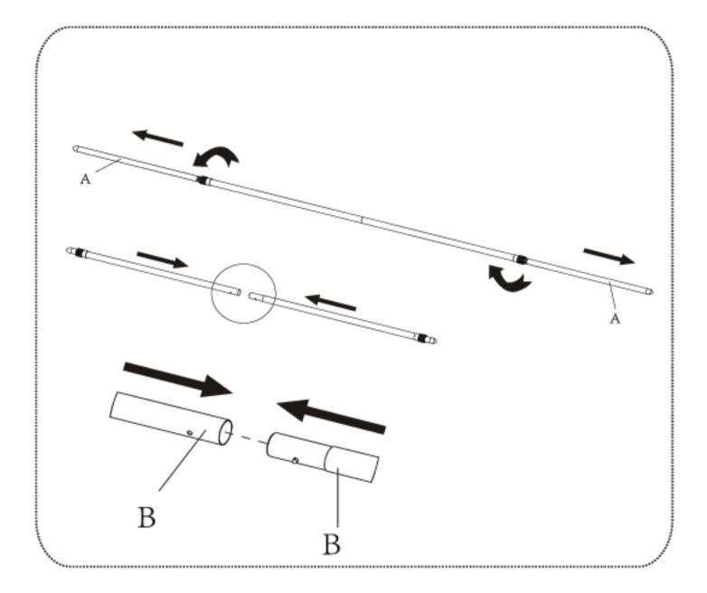
To connect B-B,pull out pole A to the tlimited stop then tighten the plastic bolt. Same way to the pole #C-D.
